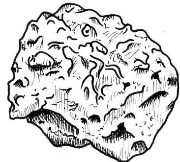
The molten appearance of a piece of iron slag
